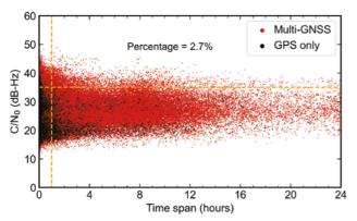
Figure 10. Distribution of time span and C/NO of collected data. Each dot represents a data file containing GNSS observations from a single session. Black dots indicate files with GPS observations only, while red dots represent files with multi-GNSS observations. The horizontal dashed line denotes the C/NO threshold of 35 dB-Hz, while the vertical line denotes the time span threshold of 1 h.
