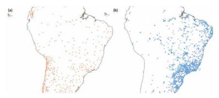
Figure 5. An example of gap filling of measurements in Brazil showing (a) publicly available GNSS stations of geodetic grade in orange and (b) data collected via the CAMALIOT app in blue.
