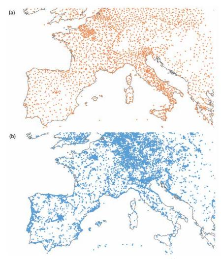
Figure 6. An example of densification of measurements in Europe showing (a) publicly available GNSS stations of geodetic grade in orange and (b) data collected via the CAMALIOT app in blue.
