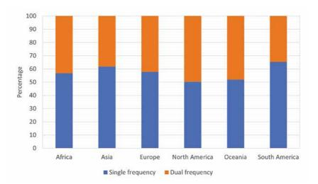
Figure 9. Continental distribution of mobile phones by single- and dual-frequency GNSS recording capabilities
